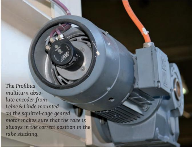
The Profibus multiturn absolute encoder from Leine & Linde mounted on the squirrel-cage geared motor makes sure that the rake is always in the correct position in the rake stacking.
